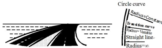
Fig. 3. Easement curve sections
