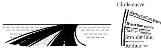
Fig. 3. Easement curve sections
